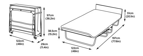
Bed weight: 31kg / 68lb Space under bed when open: 23.5cm (9.3in) Mattress dimensions: W120cm (47.2in) L191cm (75.2in) D10cm (3.9in)
